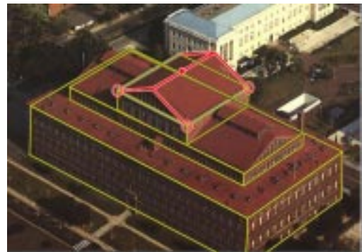
With three corners glued to the box, the roof's orientation is fixed.
